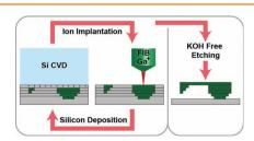
A method for additive layer-by-layer fabrication of 3D Si micro- and nanostructures is reported. The fabrication is based on alternating chemical vapor deposition of Si and local implantation of gallium ions by focused ion beam (FIB) writing. In a final step, the defined 3D structures are formed by etching the silicon in KOH, in which the local ion implantation provides the etching selectivity.
