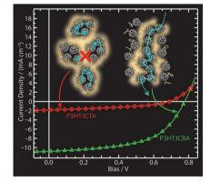
Photovoltaic devices based on a bulk heterojunction of bis-indene-C<sub>60</sub> with poly(3hexylthiophene) show enhanced power conversion efficiency due to an improved open circuit voltage. The addition of a third indene unit to form tris-indene- $C_{60}$ dramatically hinders both the local and bulk electron transport in the tris-indene-C<sub>60</sub> phase due to the formation of small, isolated tris-indene-C<sub>60</sub> clusters, resulting in poor device performance.
