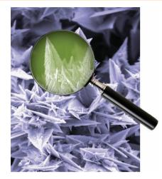
Highly porous and preferentially {100} oriented platinum nanowires and thin films ( $R_f = 500$  and up to 50% of (100) surface sites) are prepared by electrodeposition on different substrates without additives. Compared to polycrystalline Pt, there is a factor of 4 and 2.7 increase of the normalized electrocatalytic activity ( $\mu A \ cm^{-2}_{Pt}$ ) for the electro-oxidation of hydrazine and ammonia, respectively.
