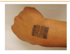
Materials and mechanics approaches are reported for an all-elastomer strain measurement device with a gauge factor as high as 29 and Young's modulus that approaches that of the human epidermis. Measurements using a system of this type laminated on the human wrist reveal that strains in the skin induced by bending of the wrist are between 11.2% and 22.6%.
