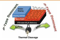
A narrow bandgap polymeric semiconductor, BOC-PTDPP, comprising alkyl substituted diketopyrrolopyrrole (DPP) and tert-butoxycarbonyl (t-BOC)protected DPP, is synthesized and used in organic field-effect transistors (OFETs). The dominant polarity of charge carriers changes from positive to negative after the thermal cleavage of t-BOC groups at 200 °C.
