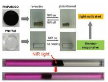
Remote Light Controlled Liquid Microvalve
